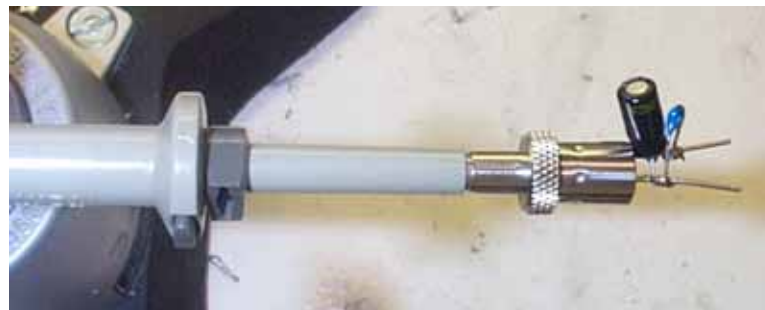
Figure 21 – Oscilloscope Probe with Probe Master 5125BA BNC Adapter (Modified with Wires for Probe Ground for Ripple Measurement, and Two Parallel Decoupling Capacitors Added).
