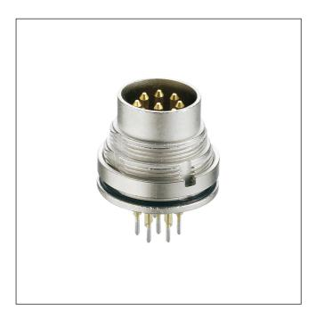
SWUM™ chassis plug acc. to IEC 61076-2-106 and AISG specification, IP 68/67, with threaded joint, for printed circuit boards, manual soldering, for rear mounting
