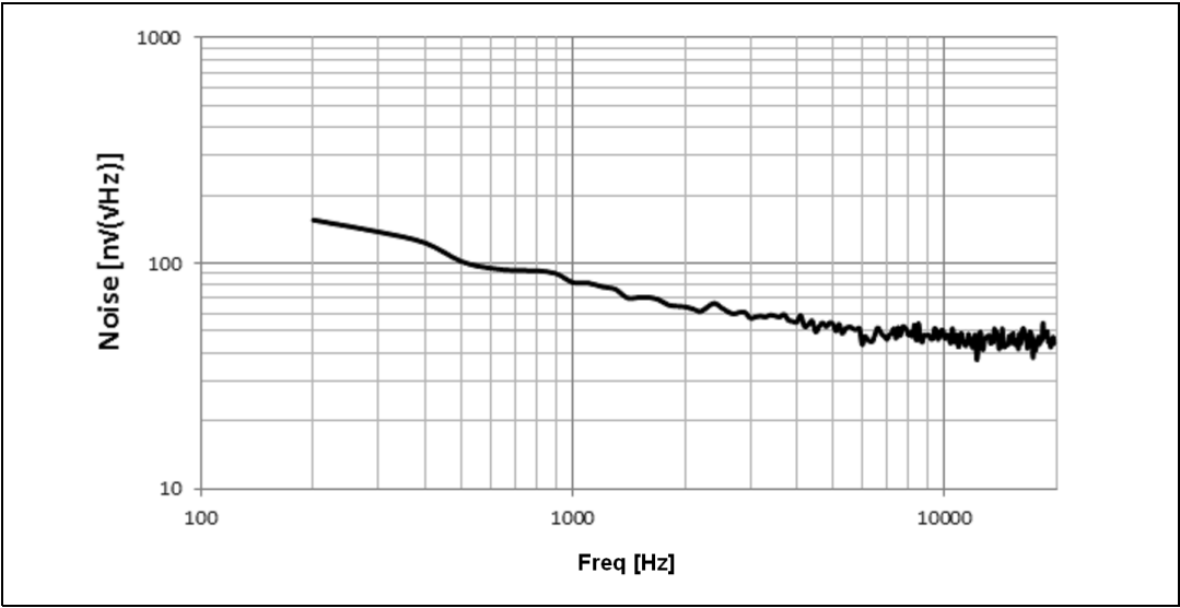
Figure 38. OPAMP voltage noise versus frequency
