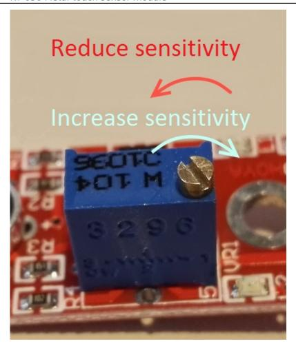
This sensor doesn't show absolute values (like exact temperature in °C or magneticfield strenght in mT). It is a relative measurement: you define an extreme value to a given normal environment situation and a signal will be send if the measurement exceeds the extreme value.
