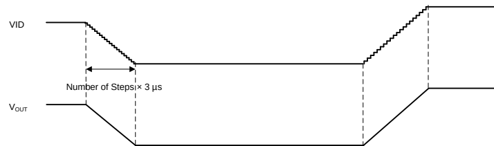
Figure 6-5. DVS Timing Diagram I
