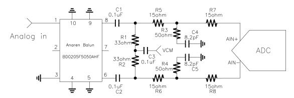
Typical ADC frontend schematic using BD0205F5050AHF
