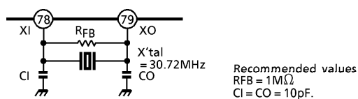
Fig.1(a) Self excited crystal oscillator
