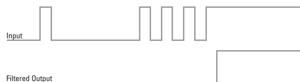
Figure 2. Debouncing and Glitch Removal
