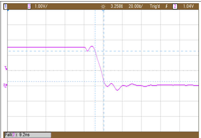
Figure 12. Fall Time of IR_TXD (Data)
