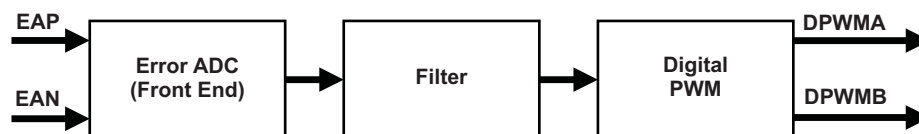
图 6-1. Simple Digital Power Configuration
