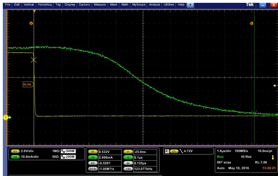
Figure: 6 Turn on time of BCR401/2/5 (PWM method shown in figure 3c)
