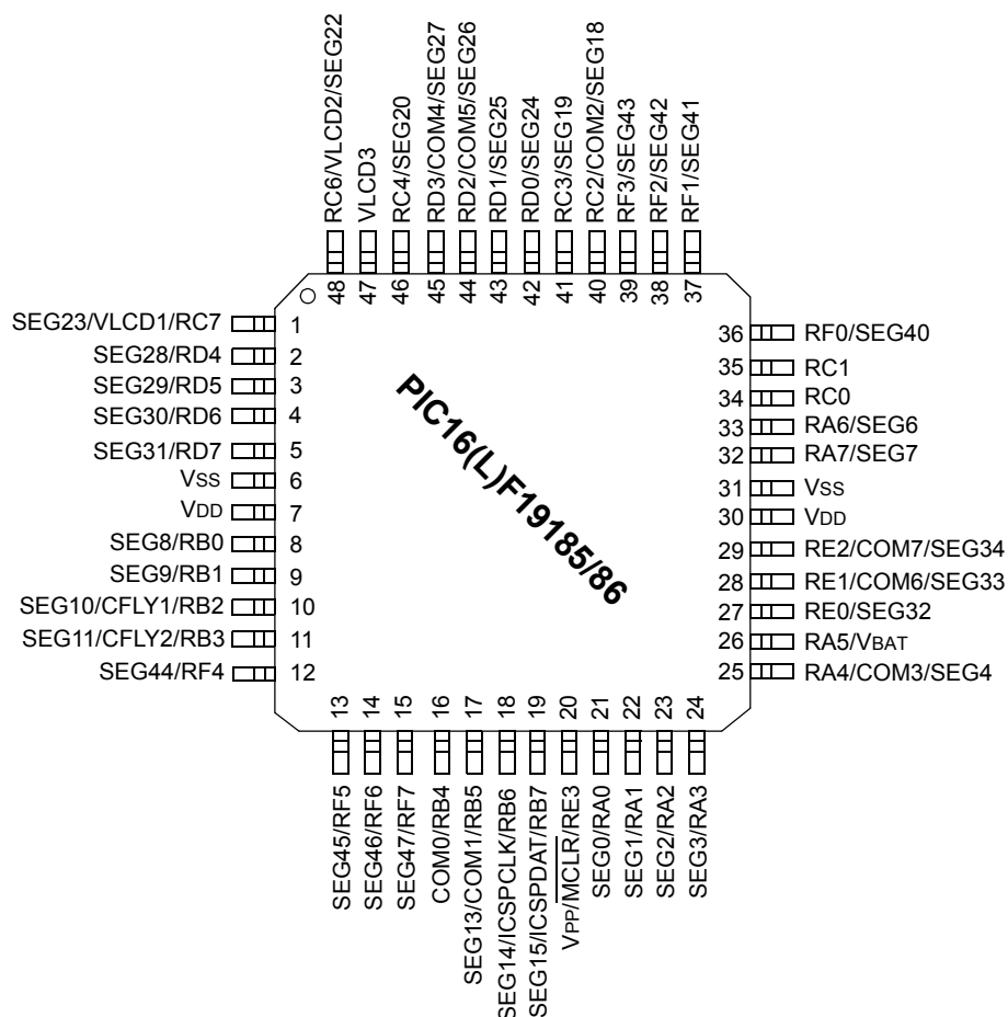
FIGURE 6: 48-PIN TQFP/UQFN PIN DIAGRAM FOR PIC16(L)F19185/86
