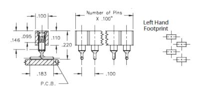
**Description:** Interconnect Socket Surface Mount Socket Accepts .015" - .025" (0,38 - 0,635 mm) dia leads
