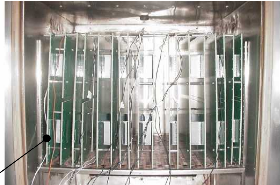
IT3-assembled test board (Refer to 4.2.2 Test board example for test board details.)
