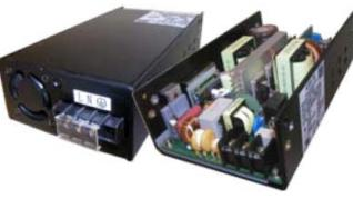
U Type (U-Chassis): 7(L) x 4(W) x 2(H) inches E Type (Enclosed with built-in fan): 8(L) x 4(W) x 2(H) inches
