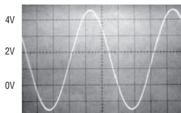
6Vp-p INPUT, -1.5\text{V} TO 4.5\text{V}
