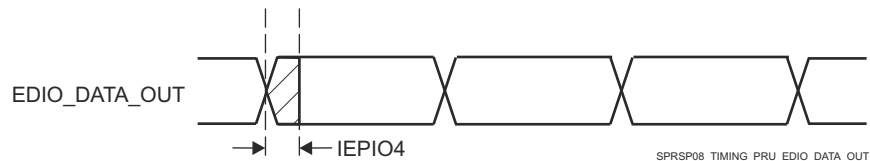
Figure 7-106. PRU_ICSSG PRU IEP Digital IOs Timing
