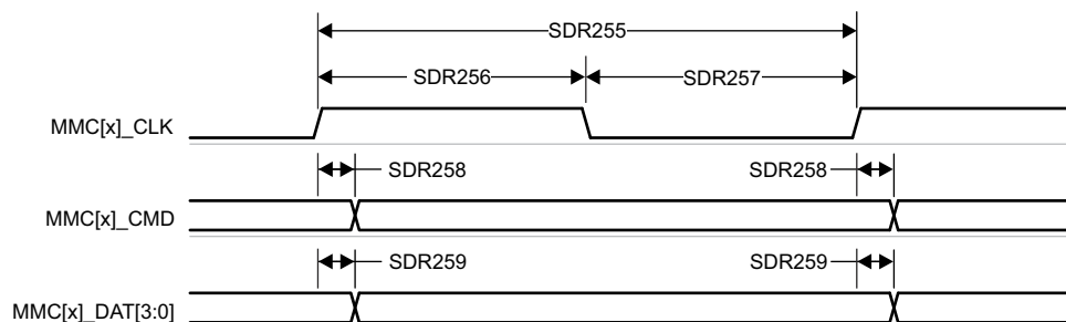
Figure 7-79. eMMC/SD/SDIO in - SDR25, 1.8-V High-Speed SDR - Transmitter Mode
