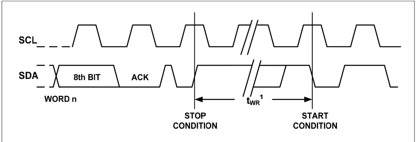
Note: 1. The write cycle time  $t_{WR}$  is the time from a valid stop condition of a write sequence to the end of the internal clear/write cycle.
