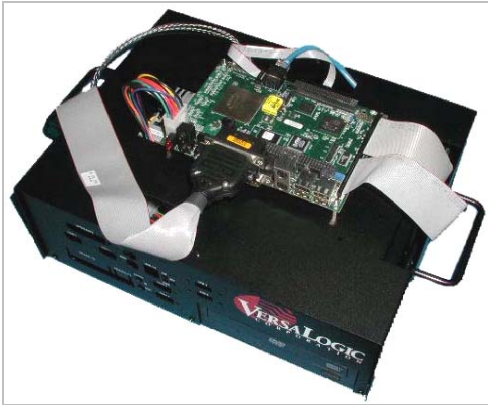
Figure 11. Example EPIC Board Installation
