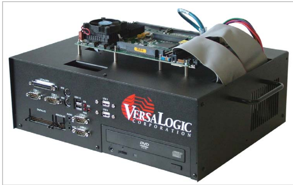
Figure 10. Example EBX Board Installation
