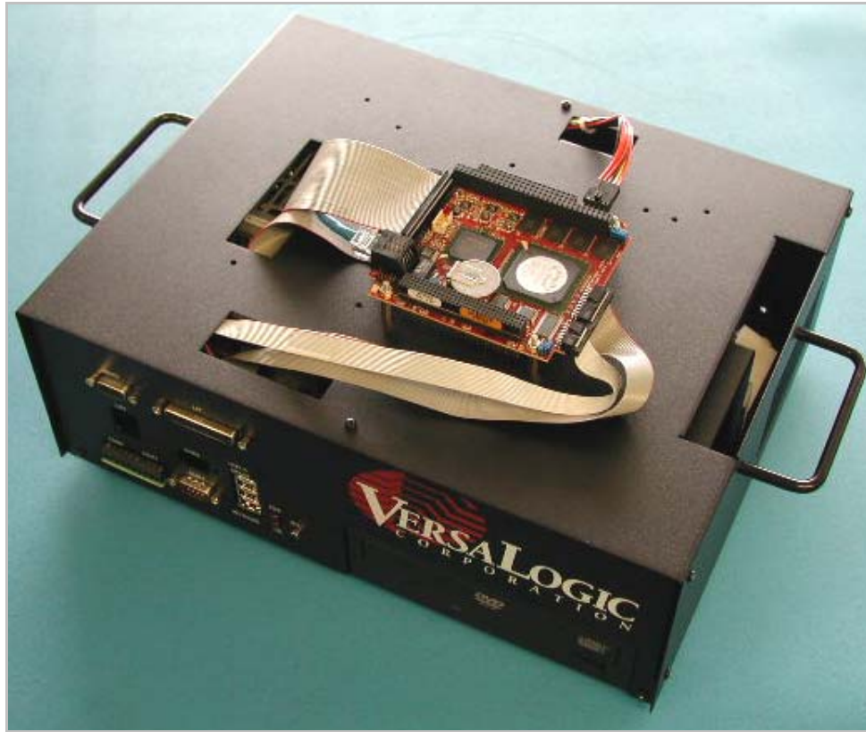
Figure 9. Example PC/104 Board Installation
