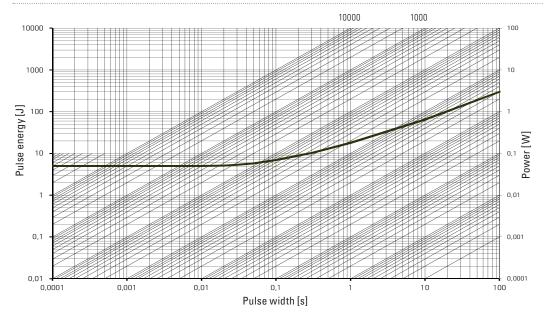
This curve is only valid for the resistance value R0003. The progression of the curve in the lower range could be different for other resistance values. Therefore a separate qualification should be made in thresholds.
