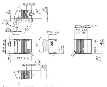
1 Blind hole thread M5, 5 mm deep (2 x), for mounting
