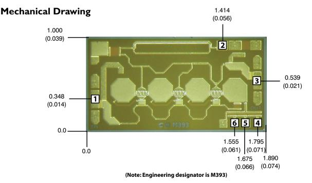
Units: millimeters (inches) Bond pad dimensions are shown to center of bond pad. Thickness: 0.076 +/- 0.010 (0.003 +/- 0.0004), Backside is ground, Bond Pad/Backside Metallization: Gold All DC Bond Pads are 0.080 x 0.080 (0.003 x 0.003). All RF Bond Pads are 0.180 x 0.080 (0.007 x 0.003). Bond pad centers are approximately 0.109 (0.004) from the edge of the chip. Dicing tolerance: +/- 0.005 (+/- 0.0002). Approximate weight: 1.172 mg
