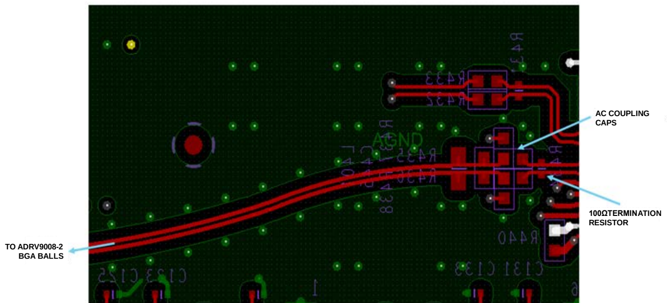
Figure 272. REF_CLK_IN \pm Routing Recommendation
