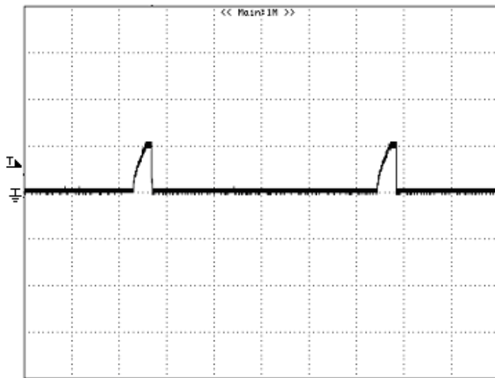
Figure 21: Output short circuit current 5V_{in} , 0.75V_{out} 20\text{A}/\text{div} , 10\text{mS}/\text{div}
