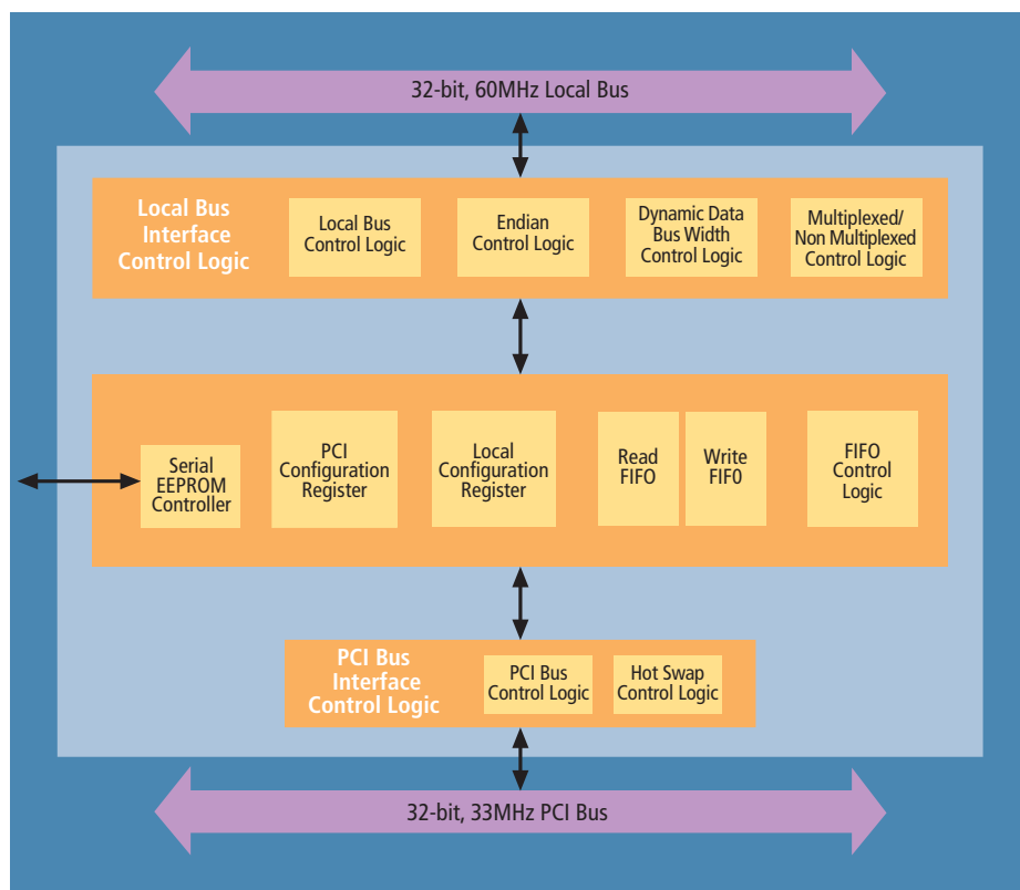
PLX PCI 9030 Block Diagram
