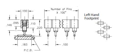
Surface Mount Socket Accepts .015"- .025" (0,38 - 0,635 mm) dia leads Single Row Surface Mount **Plating Code:** 41 Shell Plating: 200 µ" Tin (matte finish) over 100 µ" Nickel Inner Contact Plating: 10 µ" Gold over 50 µ" Nickel
