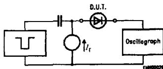
Pulse generator:  $t_p = 5 \mu\text{s}$ ,  $D = 0.05$
