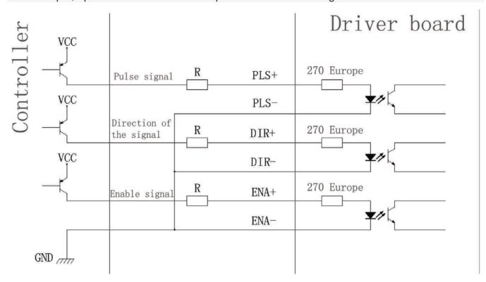
Figure 2. Input interface circuit (common cathode connection)
