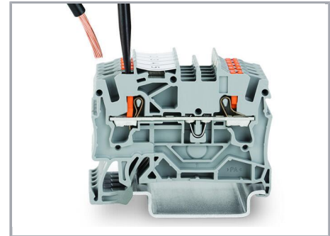
Insert fine-stranded conductors via operating tool.
