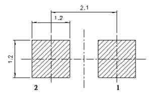
Note: Tolerances unless mentioned ±0.1mm. Unit = mm Suggested pad dimension is just for reference only. Please modify the pad dimension based on individual need.
