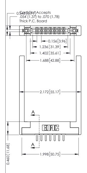
0.090[2.29] Point of Contact 305 ENG MASTER 305 / 315 / 355 Card Edge Connector J.LEE DATE: SEPT. 21/09 Part Number: 315-014-520-268 NTS SHEET 1 OF 2
