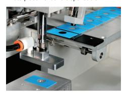
Sil-Pad® 1500ST (Soft Tack) is a fiberglass reinforced thermal interface material that is naturally tacky on both sides.
