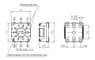
Unless otherwise specified, tolerance:  $\pm$  0.3 (Unit: mm)
