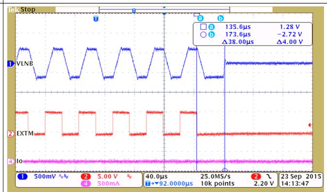
Figure 33. No load, 22-kHz Tone Delay from EXTM 22-kHz Input Turns Low to Output Tone Off
