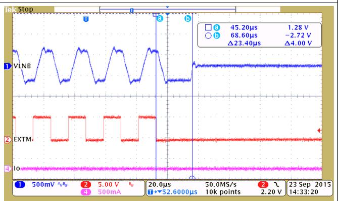
Figure 37. No Load, 44-kHz Tone Delay from EXTM 22-kHz Input Turns Low to Output Tone Off
