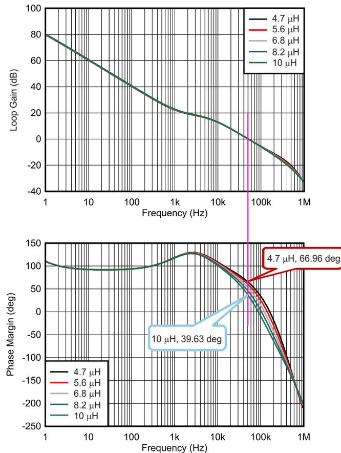
**Figure 11. Gain and Phase Margin of the Boost Loop with Different Inductance**
