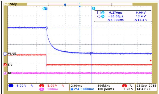
$V_{VLNB} = 13.4\text{ V}$
