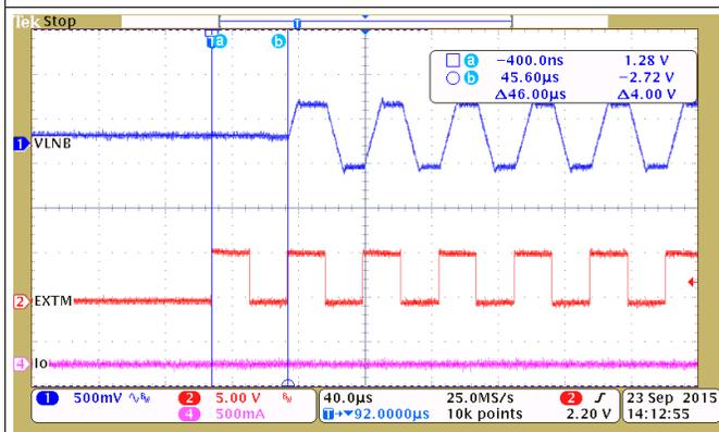
Figure 32. No load, 22-kHz Tone Delay from EXTM 22-kHz Input Turns High to Output Tone On
