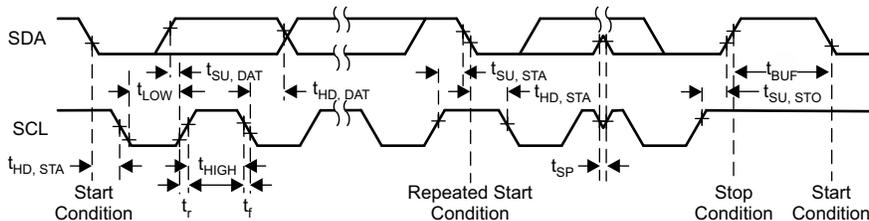
Figure 15. I<sup>2</sup>C Interface Timing Diagram
