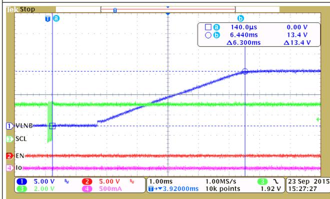
EN = 0b  $V_{VLNB} = 13.4\text{ V}$
