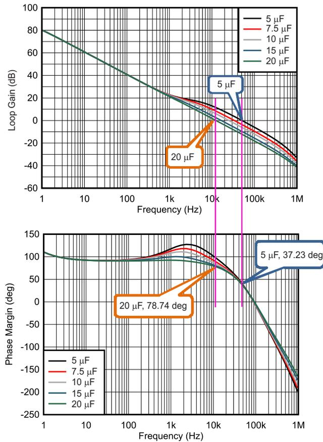
**Figure 13. Gain and Phase Margin of the Boost Loop With Different Boost Capacitance**
