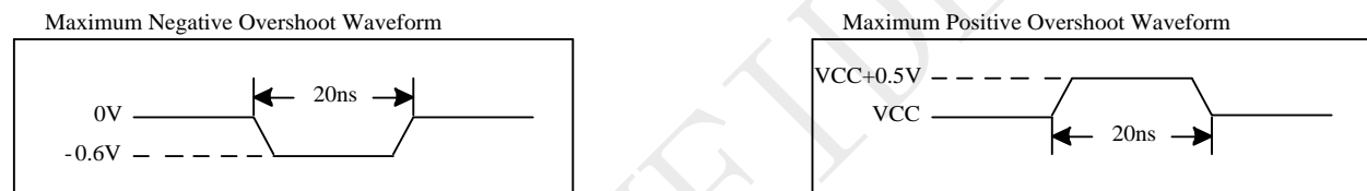
Figure 5-1 Maximum Overshoot Waveform
