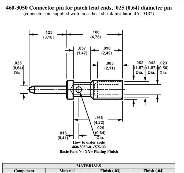
Recommended hook up wire (not supplied) 28 AWG, 7 strand x 36AWG copper wire with plastic insulation .039 (0,99) maximum diameter over insulation.
