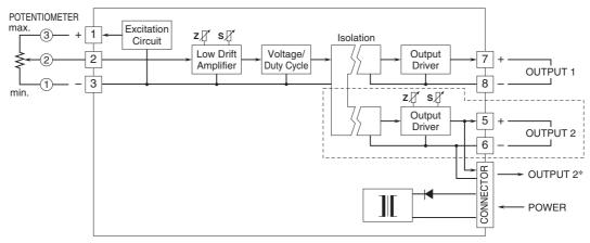
\*1 output type has the output 1 connected to the card-edge connector in parallel. Remark 1) The section enclosed by broken line is only for 2nd output channel.
