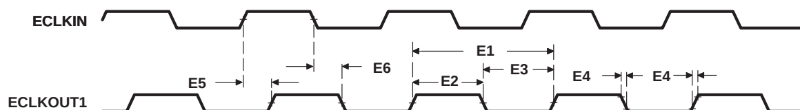
Figure 5–6. ECLKOUT1 Timings for EMIF Module
