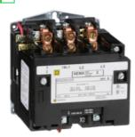
NEMA Contactor, Type S, nonreversing, Size 2, 45A, 25 HP at 575 VAC, 3 phase, up to 100 kA, 3 pole, 240 VAC coil, open
