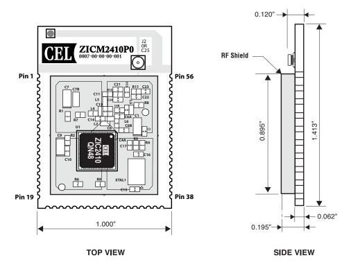
MeshConnect™ Module / MeshConnect™ Extended Range Module w/PCB Trace Antenna
