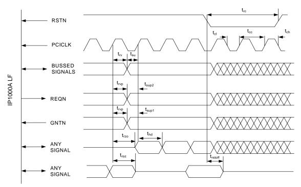
FIGURE 7-1: PCI Switching Characteristics
