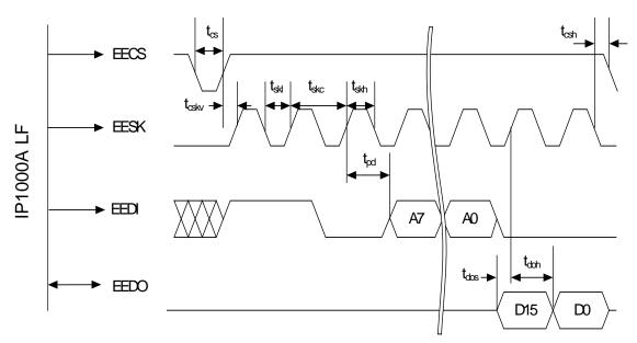
FIGURE 7-3: EEPROM Switching Characteristics
