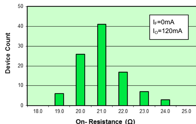
Figure 3: Typical On-Resistance Distribution (N = 100, T_a = 25^\circ\text{C} )
