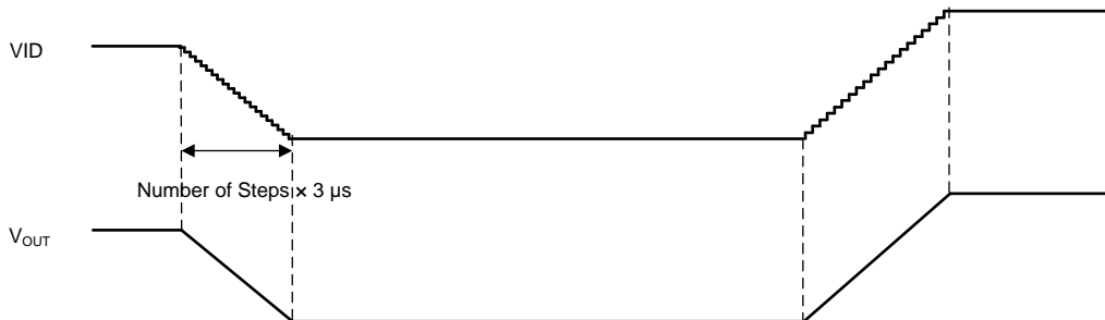
Figure 5-4. DVS Timing Diagram I (BUCKx_DECAY = 0b)
