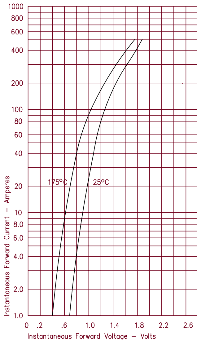
Figure 1 Typical Forward Characteristics
