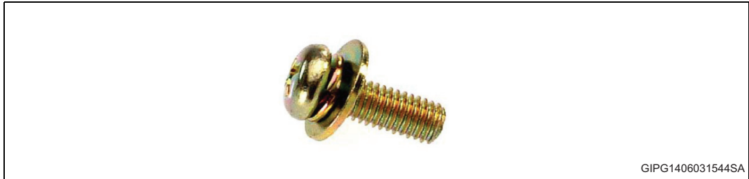
Figure 5. SEMS screw (size M3, spring washer 5.0 Φ, plain washer 7.5 Φ)
