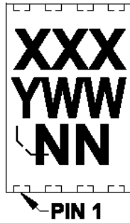
8-Lead TDFN (2 x 3 x 0.8 mm) ( MCP6V37 )
