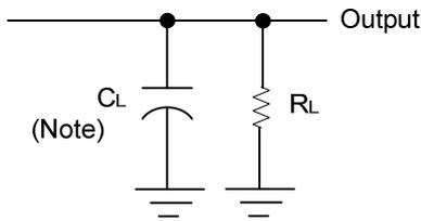
Note:  $C_L$  includes probe and jig capacitance.
