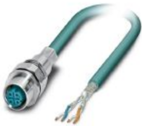
Assembled Ethernet cable, CAT5e, shielded, 2-pair, AWG 26 stranded (7-wire), RAL 5021 (water blue), M12 flush-type socket, front/screw mounting with M16 thread on free conductor end, line, length 2 m
