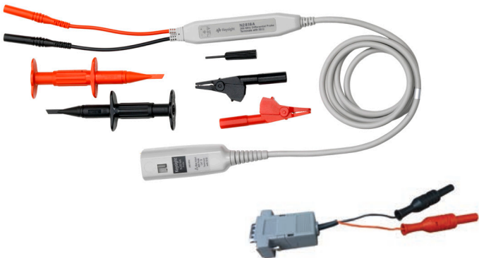
Figure 12. Keysight’s N2818A 200-MHz differential active probe.
