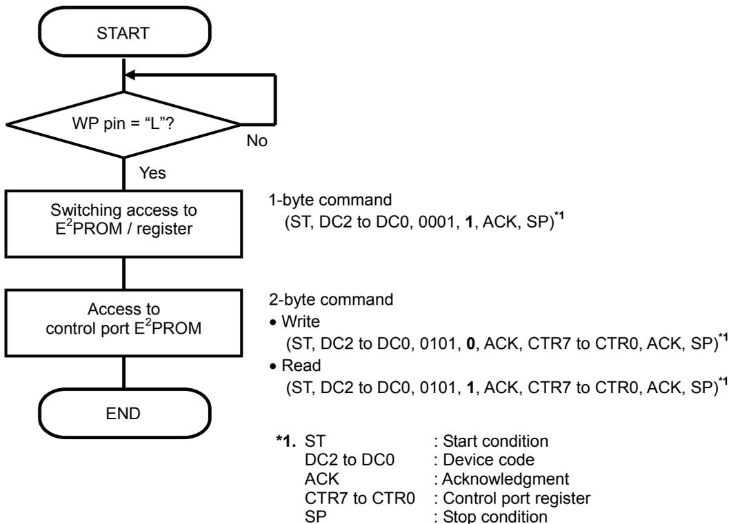
Figure 29 Flowchart for Software Example 2
