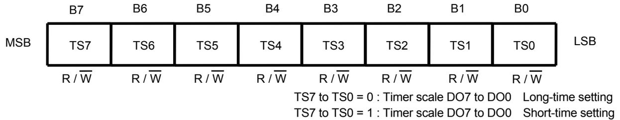
**Figure 13 Timer Scale Setting Register / E<sup>2</sup>PROM**
