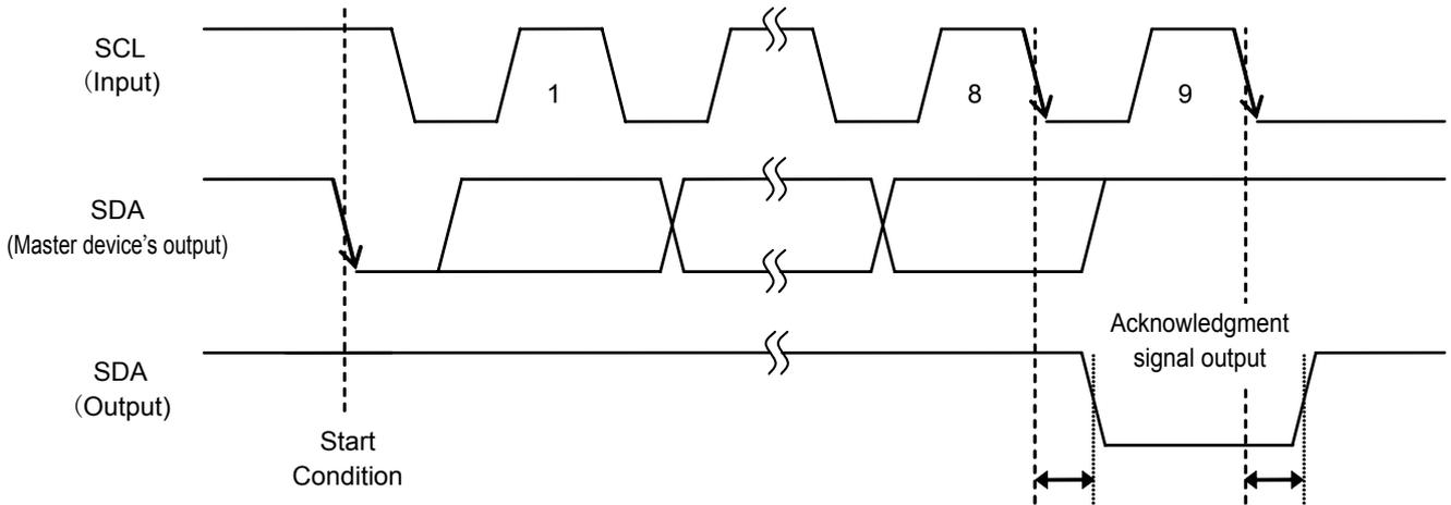
**Figure 23 Acknowledgment Output Timing 1**
