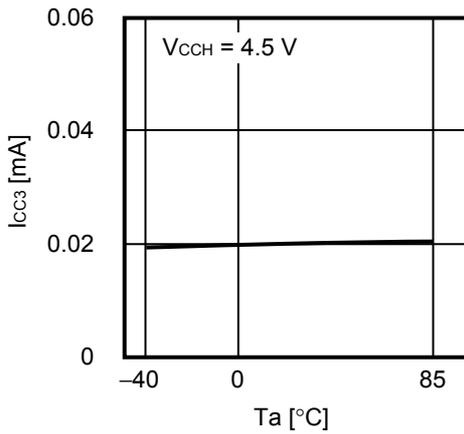
1. 10 Internal oscillator current consumption during operation  $I_{CC3}$  vs. Ambient temperature  $T_a$
