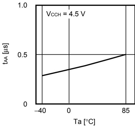
**2. 6 SDA output delay time  $t_{AA}$  vs. Ambient temperature  $T_a$**
