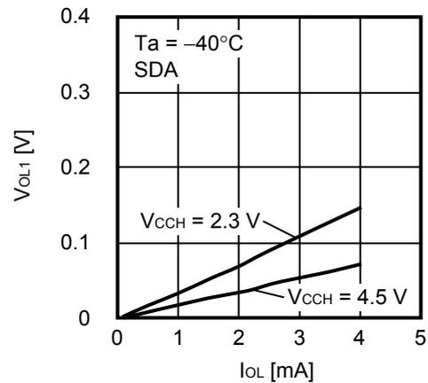
1. 19 Low level output voltage  $V_{OL1}$  vs. Low level output current  $I_{OL}$
