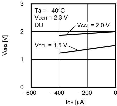
**1. 26 High level output voltage  $V_{OH2}$  vs. High level output current  $I_{OH}$**
