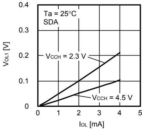
1. 20 Low level output voltage  $V_{OL1}$  vs. Low level output current  $I_{OL}$
