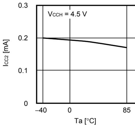
**1.6 Current consumption (PROGRAM)  $I_{CC2}$  vs. Ambient temperature  $T_a$**
