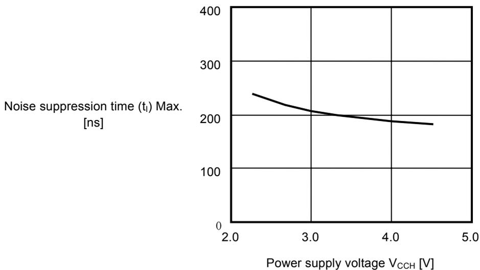
**Figure 36 Noise Suppression Time for SDA and SCL Pins**
