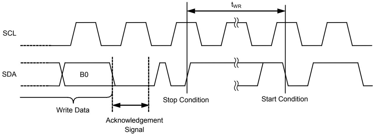
Figure 9 Write Cycle Timing
