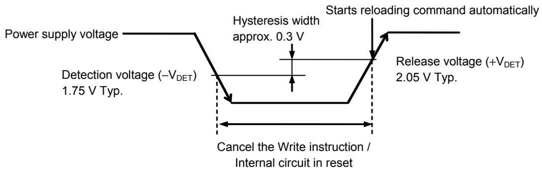
**Figure 30 Action during Low Power Voltage**
