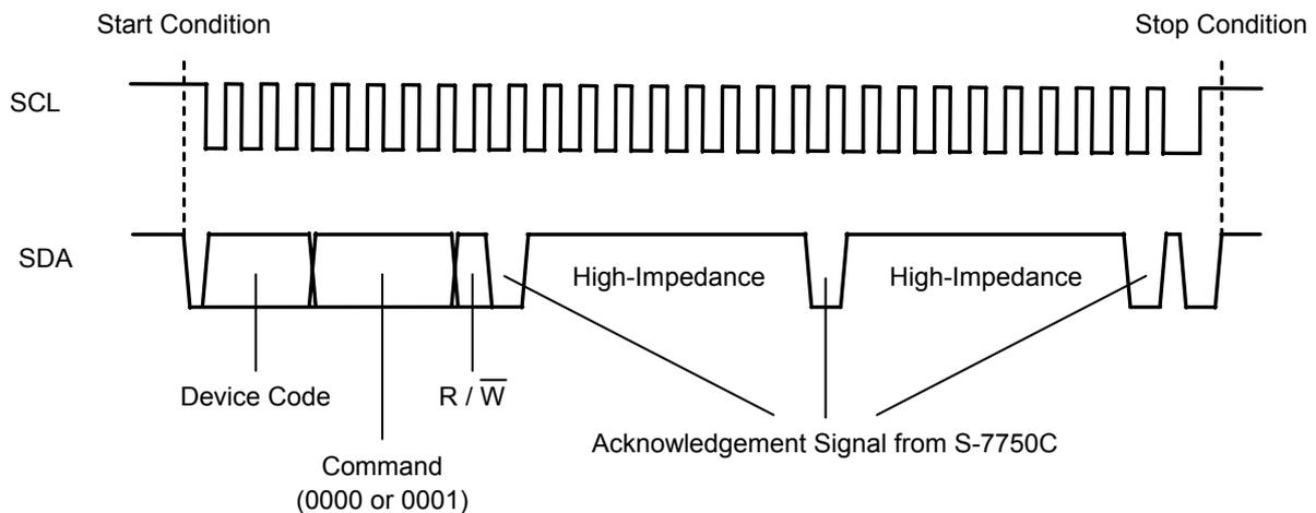
**Figure 24 Acknowledgment Output Timing 2**
