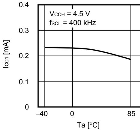
**1.2 Current consumption (READ)  $I_{CC1}$  vs. Ambient temperature  $T_a$**
