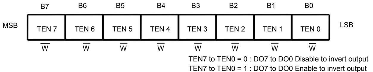
**Figure 11 Timer Enable Register**
