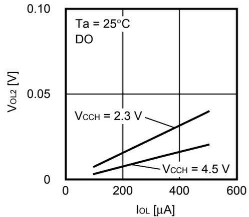
1. 23 Low level output voltage  $V_{OL2}$  vs. Low level output current  $I_{OL}$
