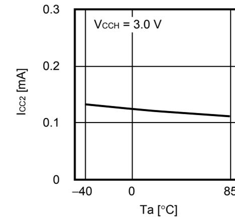
1. 7 Current consumption (PROGRAM)  $I_{CC2}$  vs. Ambient temperature  $T_a$
