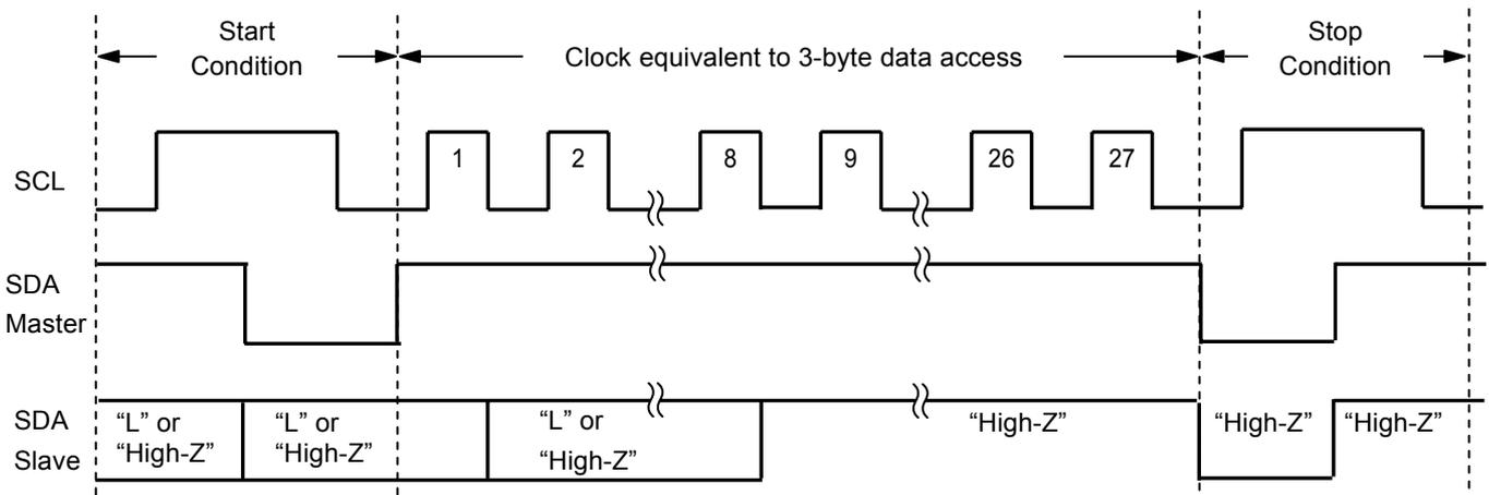
Figure 31 How to Reset S-7750C
