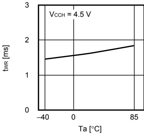
**2. 4 Write time  $t_{WR}$  vs. Ambient temperature  $T_a$**
