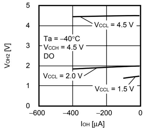
**1. 25 High level output voltage  $V_{OH2}$  vs. High level output current  $I_{OH}$**
